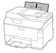
Open the feeder guard and then pinch and slide the edge guides.
